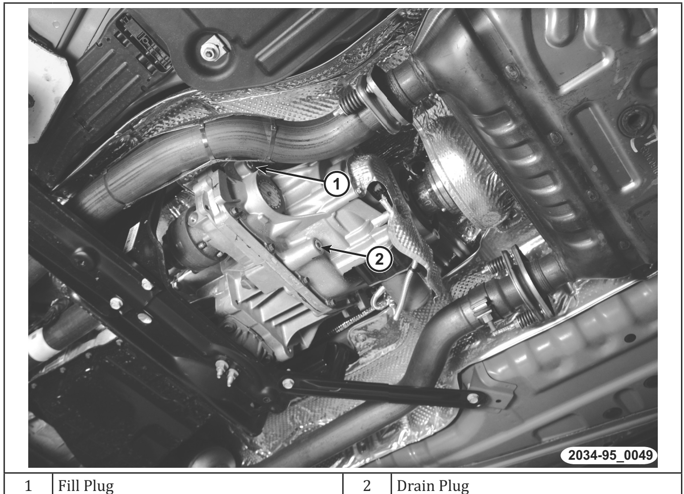
Figure 32 Drain and Fill Plug MP2010 Transfer Case Shown
