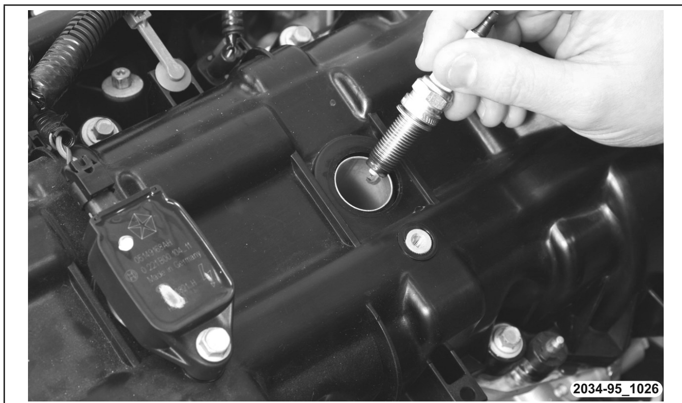
Figure 15 Spark Plug Removal/Installation
