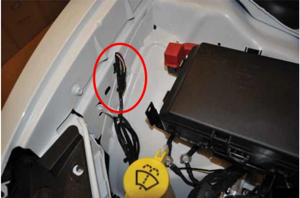
Figure 9: 12-way underhood pass-thru circuits location
